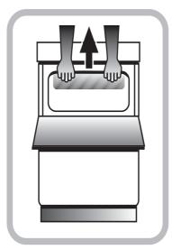
The height of the cooker can be adjusted by means of adjustable feet in the plinth (900mm - 915mm). Adjust the feet by tilting the cooker from the side. Then install the product into position. NOTE: This appliance must not be fitted on a platform.
